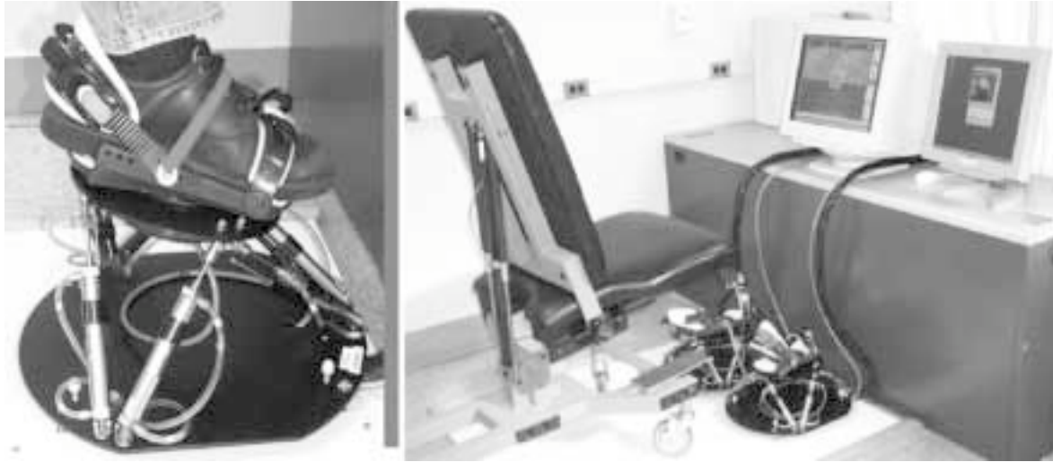
Figure 3. Rutgers Ankle Rehabilitation System. Six degrees of freedom robot on the left serves as input device for the simulation displayed on the desktop on the right. Reprinted with permission from UMDNJ and Rutgers.
